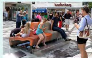
The physical prototype for the Forumtorget Bench tested the production technology, the sub-structure and three different materials for the 65 meter bench and was also deployed on site for user feedback.
